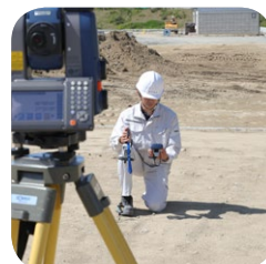
Auto-tracking test under high speed vibration conditions
