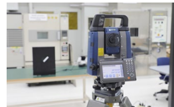
Auto-tracking durability test against rotating object.
